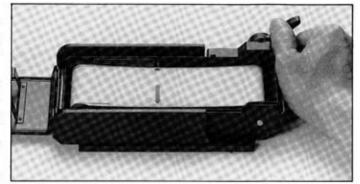
After some strokes of film advance lever, an arrow mark will be appeared on the back side of lead paper. Align the mark to the start mark located upper center of housing.
